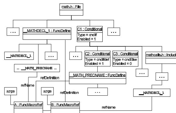
**Fig. 1.** `math.h`: example Schema instance - UML Object diagram
