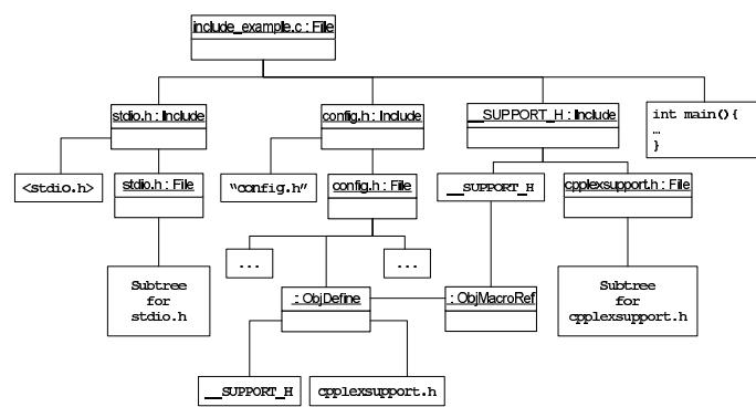
**Fig. 4.** Schema instance of the example of include directive
