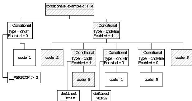
**Fig. 5.** Schema instance of the example of conditional compilation
