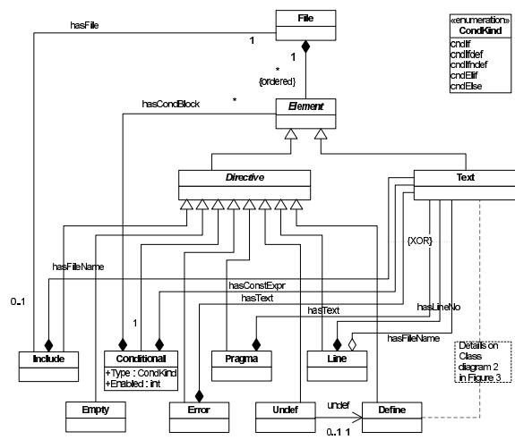
**Fig. 2.** Schema UML Class diagram - Directive part
