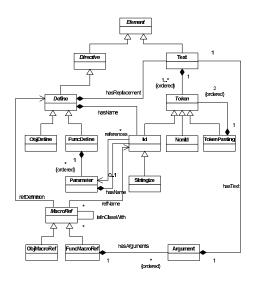
Fig. 3. Schema UML Class diagram - Text and Define part
