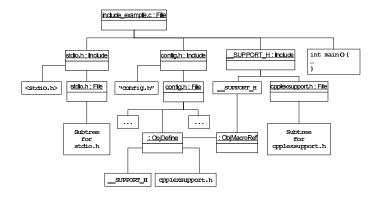
Fig. 4. Schema instance of the example of include directive  $\mathbf{F}$
